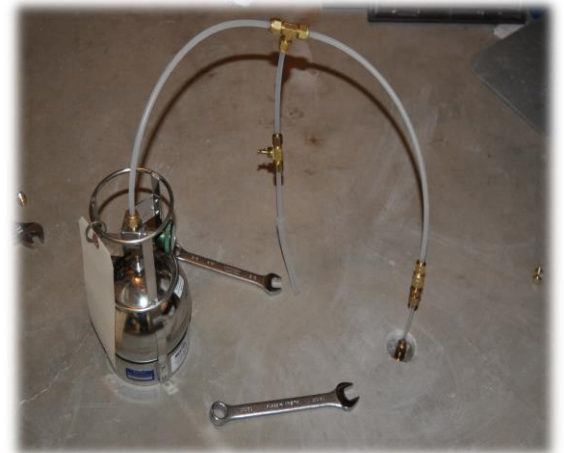
Sampling Sub-slab Vapor Monitoring Point
